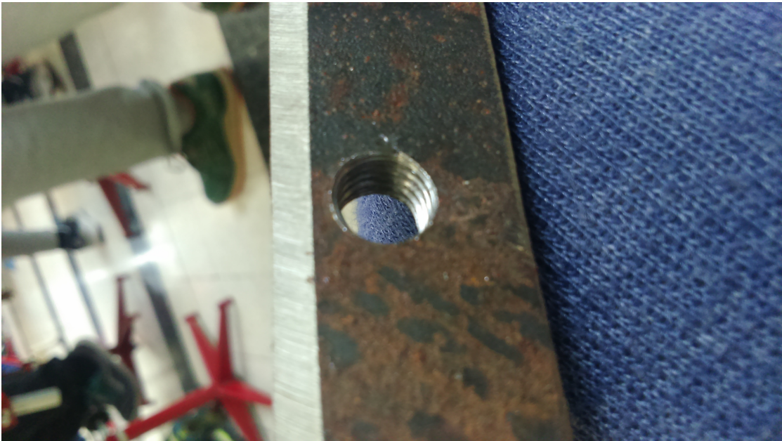
FIGURE 4.35.: Taraudage du support
